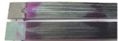
Cohesive failure specimen
